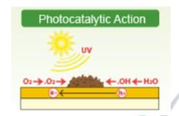
EverClean Topcoat TIO2 technology is a chemical reduction process that decomposes two atmospheric pollutants nitrogen oxide and sulfur oxide in the presence of UV light. These pollutants commonly found in exhaust fumes and smoke, are major contributors to acid rain and urban ozone. The EverClean chemical reduction process releases nitrate ions that are eventually washed into the soil and help to fertilize plants.
